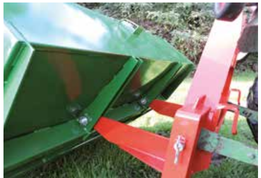
Mechanical tipping device
