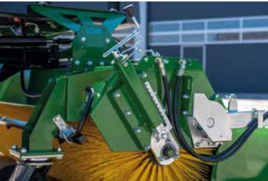
Quick brush height adjustment
