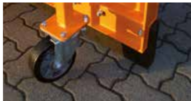
50 mm rubber strip and support wheel
