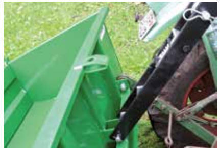
Mechanical tipping device
