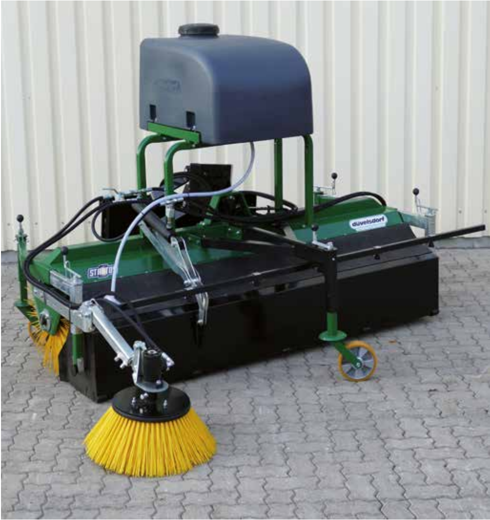
Illustration shows Stratos 1.70 m EURO, 3rd support wheel, spray equipment, hydraulic collection pan operation and a side brush PPN
