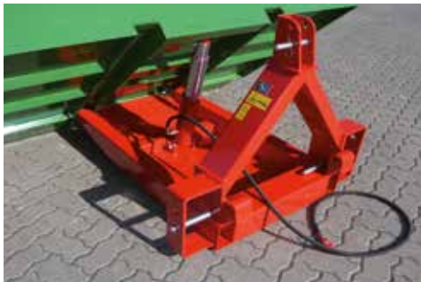
Hydraulic dump device, approx. 60° / EW
