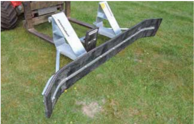
3-point attachment CAT 2 and forklift, pockets for forklift: approx. 16 x 6 cm
