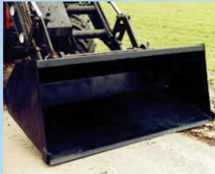
Erdschaufel 1,25 m (197 kg) 1,50 m (220 kg) 1,75 m (258 kg) 2,00 m (285 kg) 2,25 m (308 kg) 2,40 m (327 kg)
